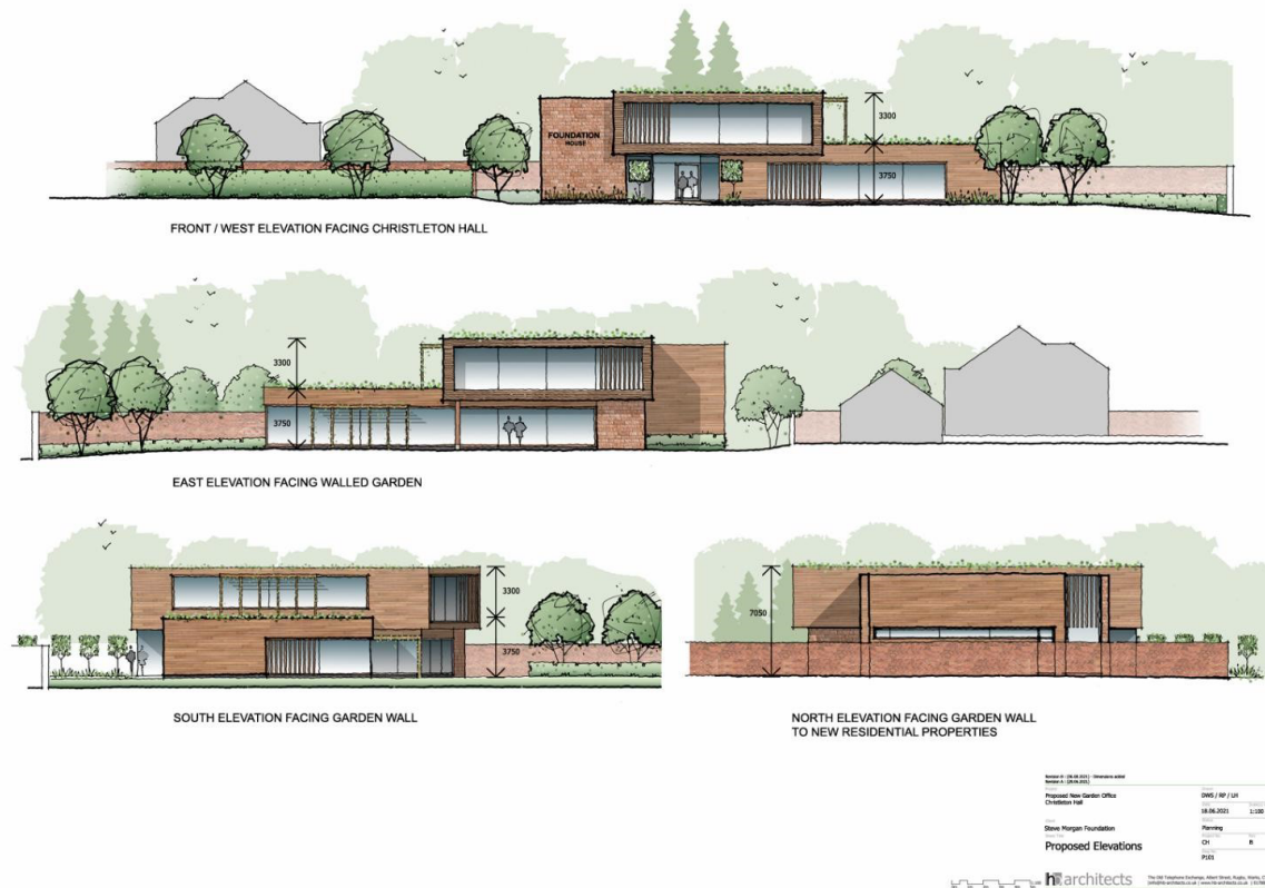
Figure 2 – Approved office building: proposed elevations
